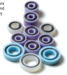
Surface finish also affects sealing ability. A rough finish creates a microscopic "line of sight" channels allowing a flow path through mating parts. When sealing gases with small molecules, such as, hydrogen, helium, or oxygen, a 2-4 Ra is highly recommended.
